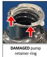
**DAMAGED** pump retainer ring
