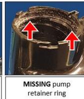
**MISSING** pump retainer ring
